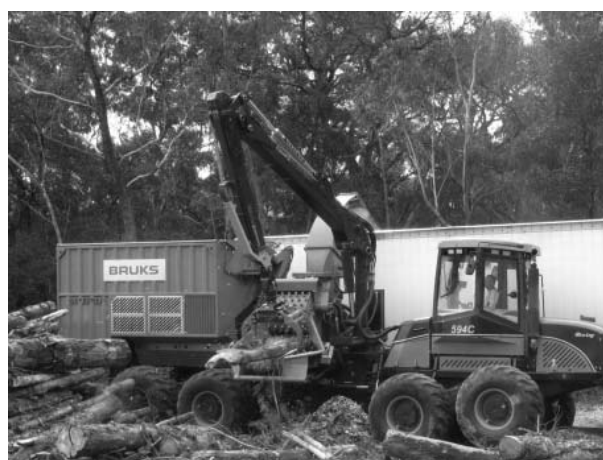
Fig. 2. Bruks mobile chipper for chipping residue piles at the roadside
