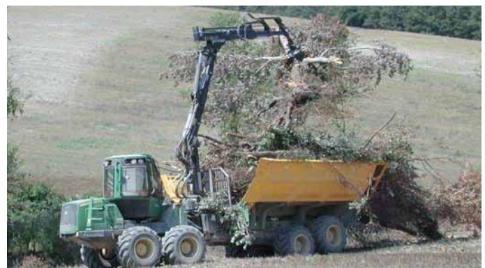
Figure 2. Biomass collector Monchiero & C. Snc
