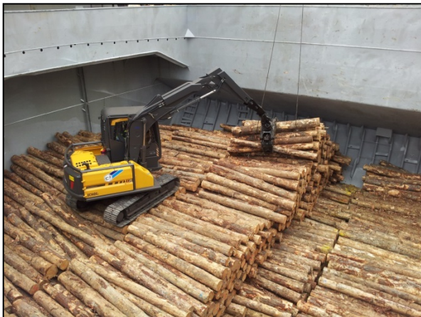
Figure 1. Most wood is exported as bulk cargo. In this figure logs are being removed from a wire sling by a small digger in the cargo hold. The digger also neatly places the logs to maximise storage volumes. (Source: C3 Ltd.)
