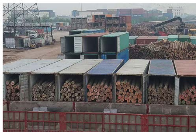
Figure 6. Huangdao Container Terminal in China showing containers that are ¾ "ful" due to 25 metric ton weight restrictions. (Source: tptforests.com)
