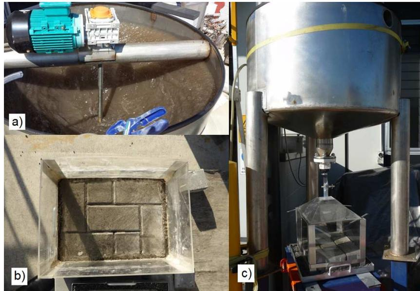
Figure 1. Accelerated Stormwater Simulation Testing Setup
