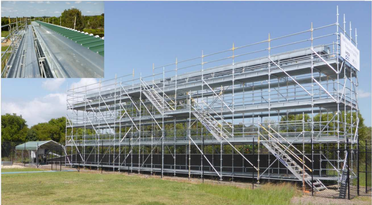
Figure 1 – Full-scale experimental roof drainage research facility at the University of the Sunshine Coast.
