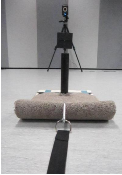
Figure 1: Carpet Attached to the Sled to Prevent Damage to the Linoleum Floor
