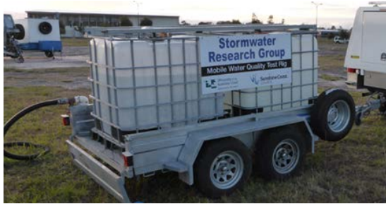
Fig.4 Stormwater supply rig used to simulate test inflow rates used in the study.
