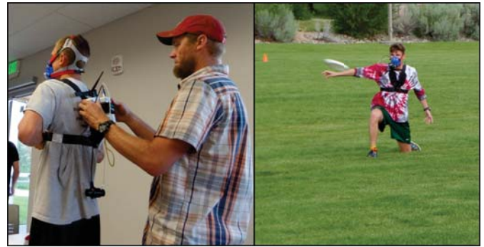
Figure 1 – The Oxycon Mobile metabolic system attached to a participant before (left) and during an Ultimate Frisbee match (right)
