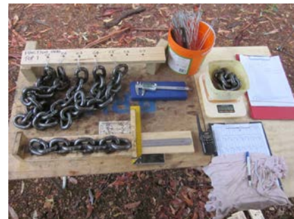
Figure 4. Chain measurement station
