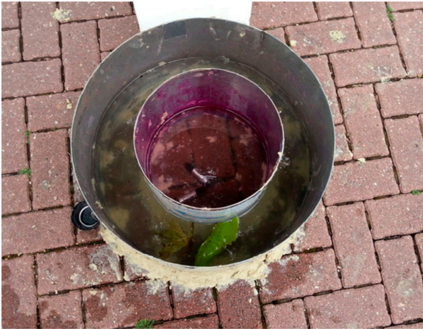
Figure 6. Middle double ring infiltrometer test (two minidivers can be seen in middle ring).
