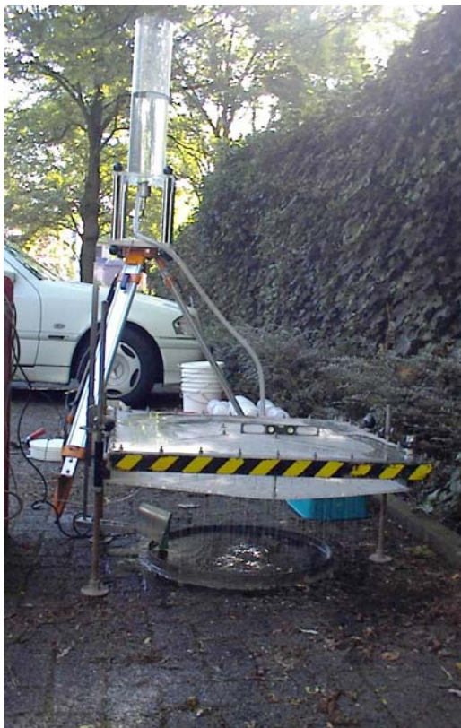
Figure 6 - Test Rig for Rain Simulation Testing (Dierkes et al., 2002)
