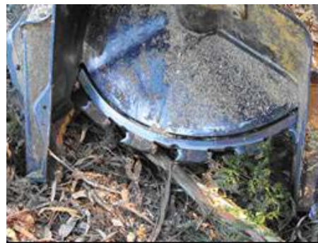
close-up of hot-saw head (right)
