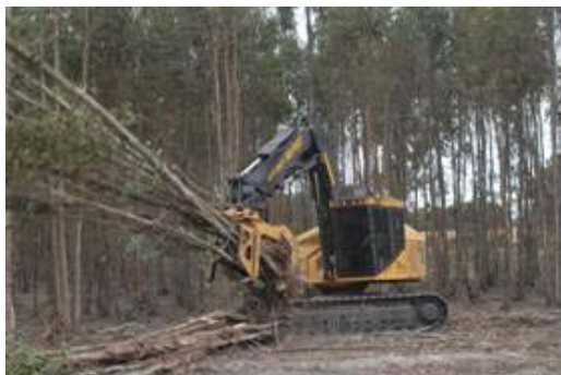
Feller-buncher harvesting blue gum plantations (left);
